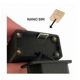
The device is intended for listening to conversations from a room over very long distances. The device operates on the principle of GSM network, and for its normal operation it is necessary to ensure a normall SIM card. The location where the device will operate must be covered by a GSM signal (check with a regular cell phone).
